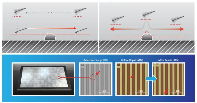
Photomask defects are a result from foreign particles in the environment or by erroneous pattern processing. The most commonly found defects on high-end photomasks are tin particles generated during the lithography process. The AFM nanomechanical method of Park NX-Mask offers many advantages that are superior and completely safe for photomask repairs.
